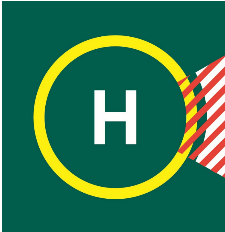
Figure 6: Example of prohibited landing heading marking
